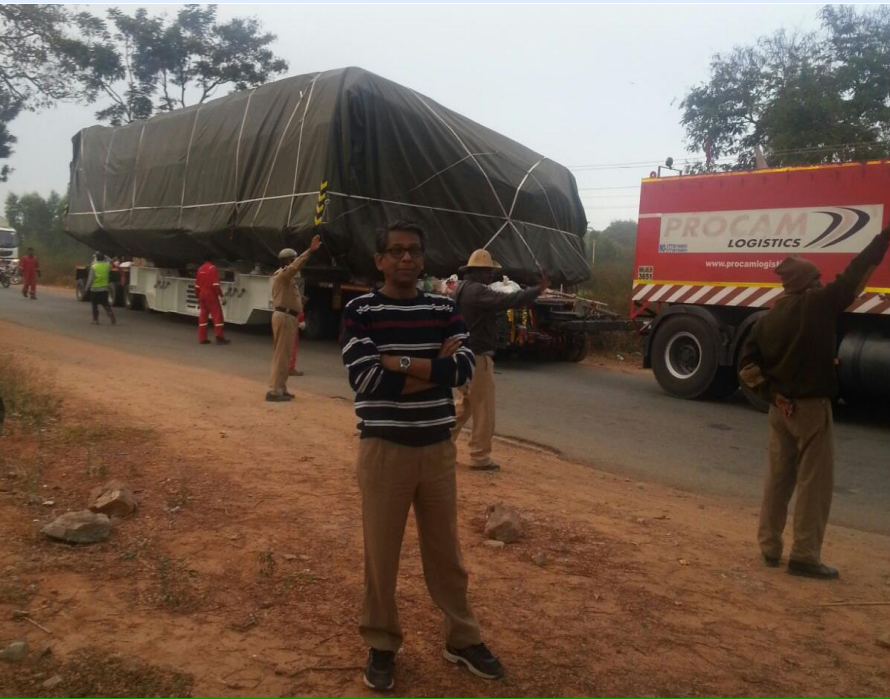
Logistics, Bangalore successfully executed the inland transportation of a huge antenna of DRDO, weighing 104 MT with a dimension of 14m x 5m x 5m from Bangalore to Kolar.
